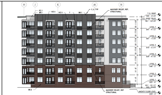
E16 BUILDING ELEVATION - SOUTH 1/16" = 1'-0"
