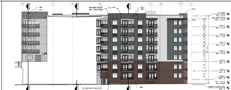
E7 BUILDING ELEVATION - SOUTH 1/16" = 1'-0"
