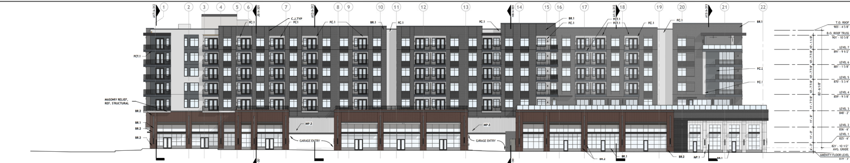
J1 BUILDING ELEVATION - WEST 1/16" = 1'-0"
