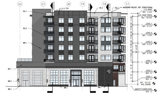
A1 BUILDING ELEVATION - EAST 1/16" = 1'-0"
