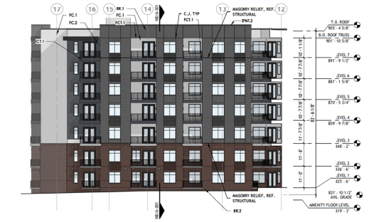
A7 BUILDING ELEVATION - EAST 1/16" = 1'-0"
