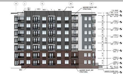
E16 BUILDING ELEVATION - SOUTH 1/16" = 1'-0"
