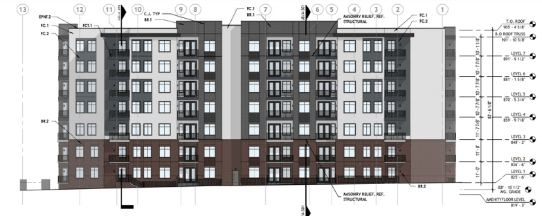
A12 BUILDING ELEVATION - EAST 1/16" = 1'-0"
