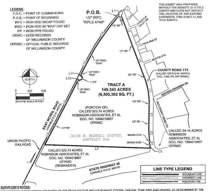
THE BEARINGS SHOWN HEREON ARE BASED ON THE TEXAS STATE PLANE COORDINATE SYSTEM, CENTRAL ZONE (FIPS 4203) (NAD'83), AS DETERMINED BY THE GLOBAL POSITIONING SYSTEM (GPS). ALL DISTANCES SHOWN HEREON ARE ON THE SURFACE. TO CONVERT SURFACE DISTANCES TO THE GRID, APPLY THE COMBINED SURFACE TO GRID SCALE FACTOR OF 0.9998881092209.THE UNIT OF LINEAR MEASUREMENT IS U.S. SURVEY FEET. A METES & BOUNDS DESCRIPTION AND A LINE & CURVE TABLE WERE CREATED IN CONJUNCTION WITH THIS TRACT BOUNDARY EXHIBIT.
