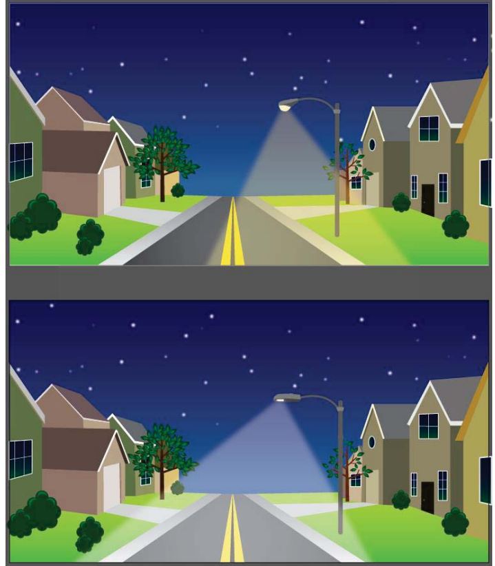
Examples of the different light distribution patterns from an HPS fixture (top) vs. an LED fixture (bottom).
