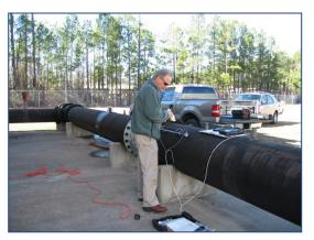
In this regard, JBS will conduct accuracy tests on the source water meters that determine the volume of water received and the costs to provide that water.
