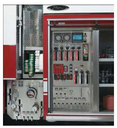
and systematically organized. The upper section will contain the master gauges. This section will be angled down for easy visibility. The center section will contain the pump controls aligned in two horizontal rows. The pressure control device, engine monitoring gauges, electrical switches, and foam controls (if applicable) will be located on or adjacent to the center panel, on the side walls for easy operation and visibility. The lower section will contain the outlet drains.
