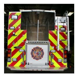
The hose bed will be directly above the rear compartment door. The dimension from the ground will be approximately 67.00" depending on the suspension and equipment load.
