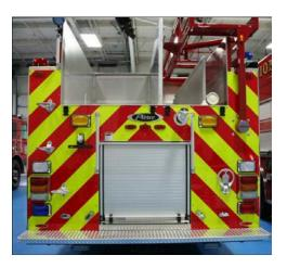
Rear compartment will be open into the rear side compartments. The transverse opening will be a minimum of approximately 22.00" wide x 27.75" high.
