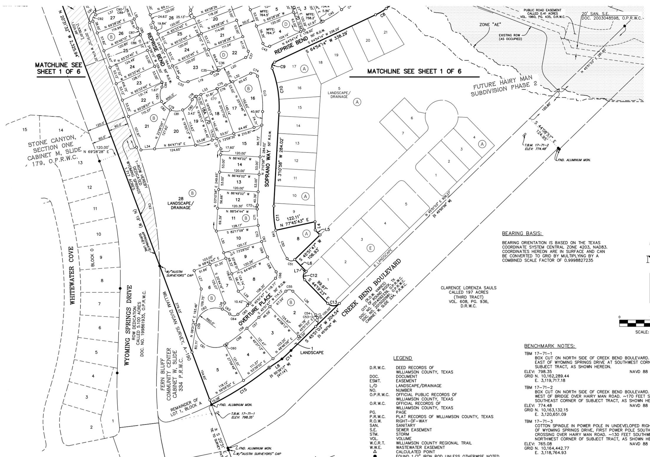
BEARING BASIS: BEARING ORIENTATION IS BASED ON THE TEXAS COORDINATE SYSTEM CENTRAL ZONE 4203, NAD83. COORDINATES HEREON ARE IN SURFACE AND CAN BE CONVERTED TO GRID BY MULTIPLYING BY A COMBINED SCALE FACTOR OF 0.9998627235
