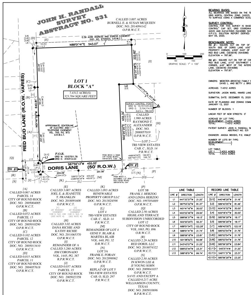
BEARING BASIS: ALL BEARINGS ARE BASED ON THE TEXAS STATE PLANE COORDINATE SYSTEM, GRID NORTH, CENTRAL ZONE, (4203), NADB3, ALL DISTANCES WERE ADJUSTED TO SURFACE USING A COMBINED SCALE FACTOR OF 1.000118481546.
